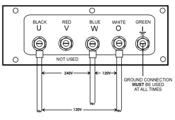
Figure 30. Output Terminal Lugs 1Ø-240V/120V Connections
